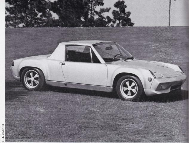
The newly designed front air dam reduced frontal lift at high speed. Fitted with the strongest engine available at the time, the 2.4-liter 911S powerplant, the 916 reached 60 mph in less than seven seconds.
